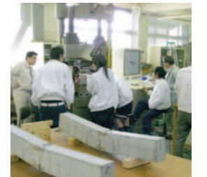
Experiment on a Concrete Beam Subjected to Bending
