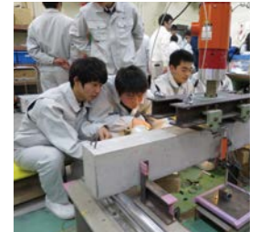
Loading of Reinforced Concrete beam
