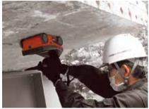
Non-destructive inspection by electromagnetic wave radar
