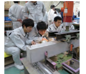
Loading of Reinforced Concrete beam
