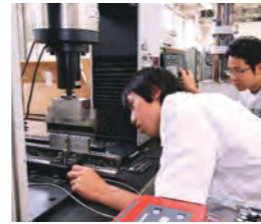
Bending Test of Metallic Materials
