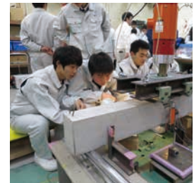
Loading of Reinforced Concrete beam
