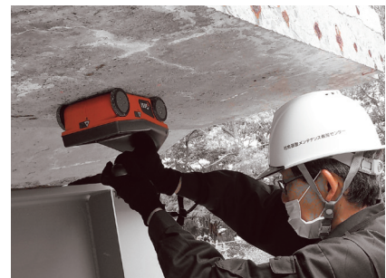
Non-destructive inspection by electromagnetic wave radar
