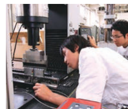
Bending Test of Metallic Materials
