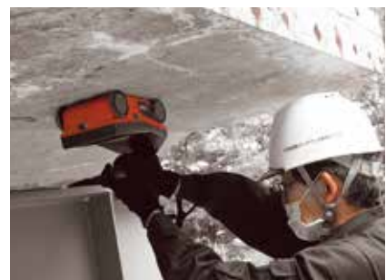
Non-destructive inspection by electromagnetic wave radar
